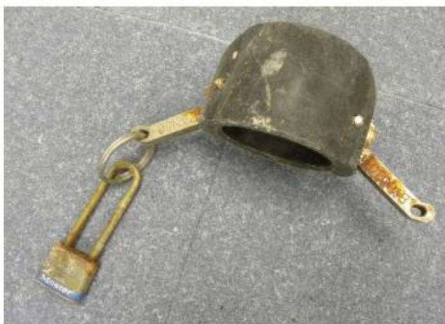
Figure 7. Sodium hypochlorite dust cap with missing split ring. The missing split ring prevented the dust cap from being secured by the padlock (Source: CSB).
