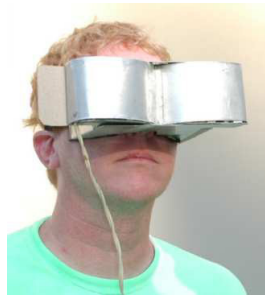
Σχήμα 2.2: Telesphere Mask, a head-mounted display (HMD), a non-interactive film medium without motion tracking
