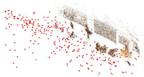
Figure 1. Point cloud and camera poses (indicated with red pyramids) reconstructed with uLF-SfM from 303 views of an indoor scene captured by Lytro Illum.
